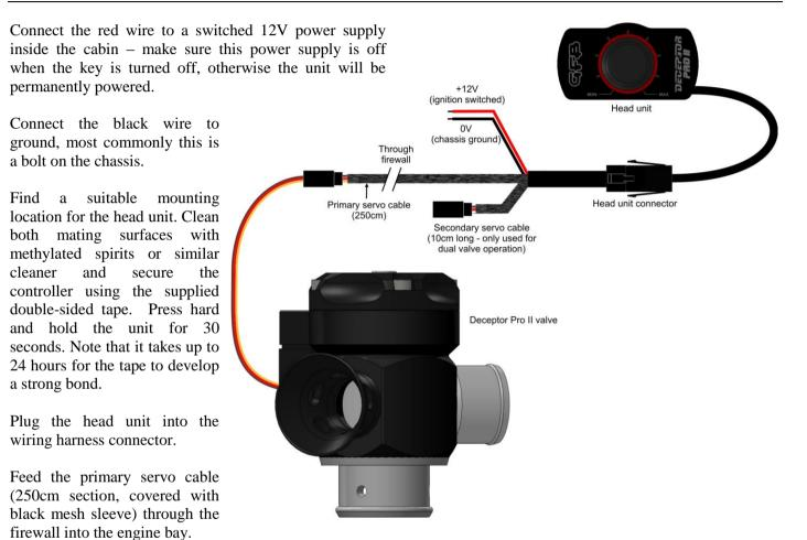
Often there is an existing grommet that can be used for this purpose. In any case, it is important to ensure that the lead is protected where it passes through the firewall to prevent wear or damage.
