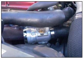
6. Connect the servo cable to the servo motor located on the side of the Deceptor Pro II valve, then secure the cable out of the way so that it does not rub or contact hot parts such as the exhaust manifold.
